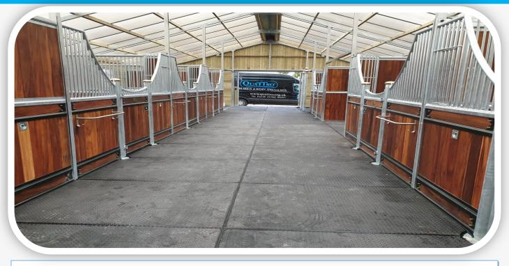
Quattro developed the Bonded & Sealed matting system over 20 years ago to alleviate the problem of urine, bedding and dirt getting under loose fitted mats which can make stables unhygienic and cause strong odours plus lifting mats in and out of stables to clean underneath is extremely difficult.
