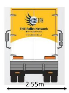
Payload is 9 tonnes. Tail-lift weight max. 1000kg
